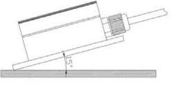
The angle between sensor and horizontal level should be about 15°.
